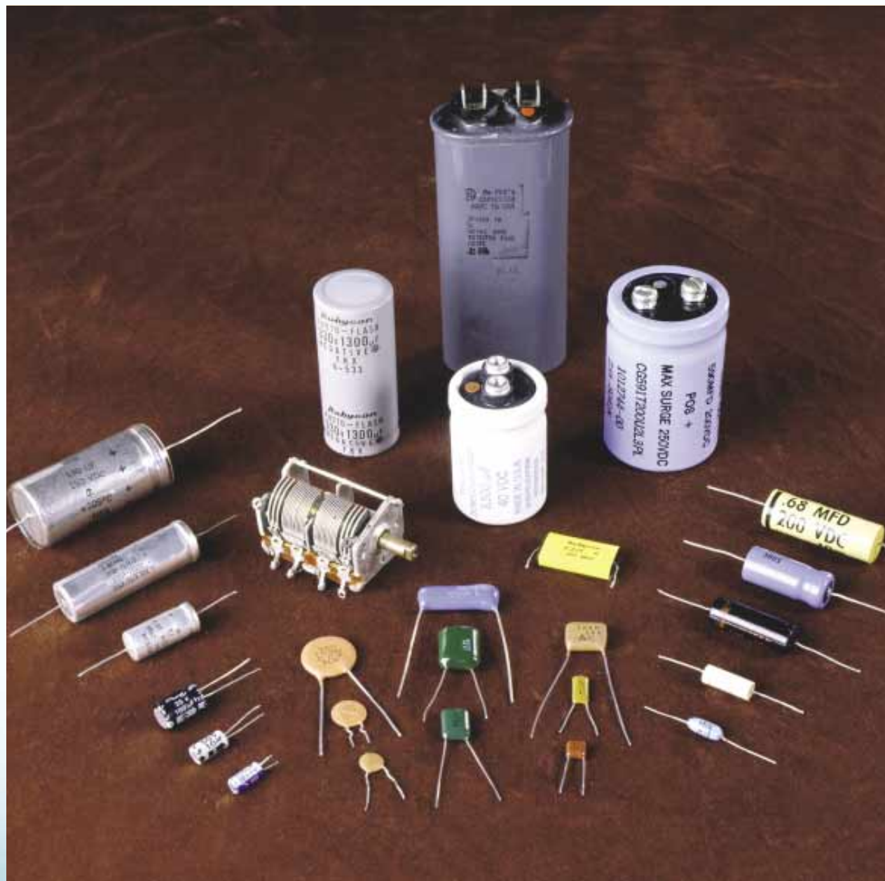
▲ All of these devices are capacitors, which store electric charge and energy. A capacitor is one type of circuit element that we can combine with others to make electric circuits. (Paul Silverman/Fundamental Photographs)
