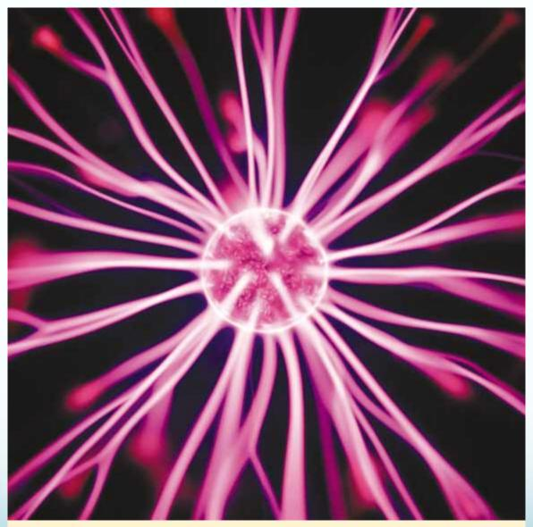
▲ In a table-top plasma ball, the colorful lines emanating from the sphere give evidence of strong electric fields. Using Gauss's law, we show in this chapter that the electric field surrounding a charged sphere is identical to that of a point charge. (Getty Images)
