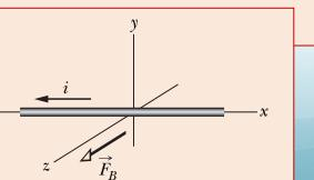
4. In a certain electric motor wires that carry a current of 8 A are perpendicular to a magnetic field of 50 mT. Calculate the magnetic force on each centimeter of these wires. Solution
